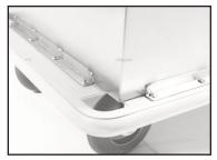
FULL PERIMETER BUMPER ... All aluminum with non-marking gray vinyl insert to protect cart and facility walls. Reinforced with angle brackets and bolted on to cabinet.
