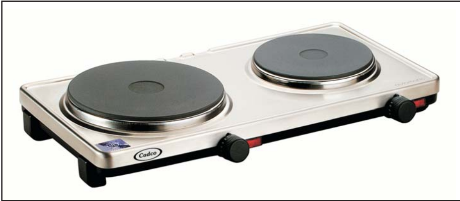
Model DKR-S2 - Double Cast Iron Range One 7 3/8" cast iron element / 1000W; one 6" cast iron element / 650W
