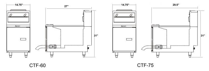
Legs are adjustable 4-5" Legs are removable and unit can sit flush on a flat surface
