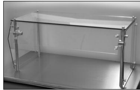
Maximum Front Glass Opening is 13" From Table to Bottom of Glass Max. load for Top Glass is 100 lbs. even dist. wt. (shown with 1" Anodized Aluminum Posts)
