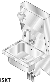
Model HSKT Includes Faucet, Basket, P-Trap, Knee Valves, Soap & Towel Dispenser, Gooseneck Spout, w/Overflow
