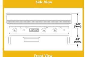
Current construction on 24", 36" and 48" wide griddles are 1/2" taller than indicated in drawing. Current construction subject to change. Contact factory for current dimensions if required.
