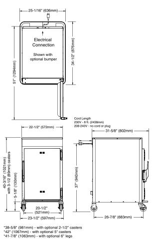
**DIMENSIONS:** H x W x D **EXTERIOR:** 40-3/16" x 22-1/2" x 31-5/8" (1021mm x 572mm x 802mm) **INTERIOR**: 26-7/8" x 18-7/8" x 26-1/2" (683mm x 479mm x 673mm)
