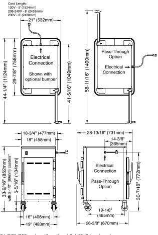
\*31-7/8" (809mm) - with optional 2-1/2" (64mm) casters \*35-1/4" (895mm) - with optional 5" (127mm) casters \*33-15/16" (861mm) - with optional 6" (152mm) legs
