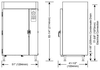
Legs not installed at factory
