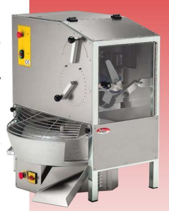
The BakeMax® Dough Divider Rounder combo can divide dough from approx. 50 to 650 gram portions and round the divided dough into the perfectly sized dough ball each time.
