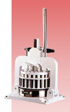
Divider manually divides dough into 36 equal dough balls. Size of dough balls approximately
