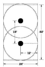
\*Note: Ambient temperatures and wind conditions vary and will affect heater performance. To maximize layout distances, employ building walls, alcoves, fences and shrubbery lines as wind barriers.
