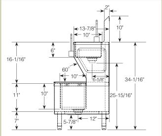
This unit can be plumbed in the field to a floor drain if available or to a 1-1/2" drain pipe. 1/2" MPT for cold water connection only with less than 45 psi.
