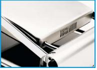
**Compact System:** The electrical connections of the covers pass through a metal tube inside the body of the appliance. This patented design greatly reduces overall dimensions and allows the grill to be positioned against the wall.
