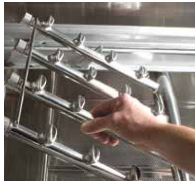
One-Piece Cast Stainless Steel Spray Assembly
