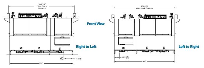
NOTE: For complete machine dimensions, plan view, end view, specifications and table construction see 64 drawing page.
