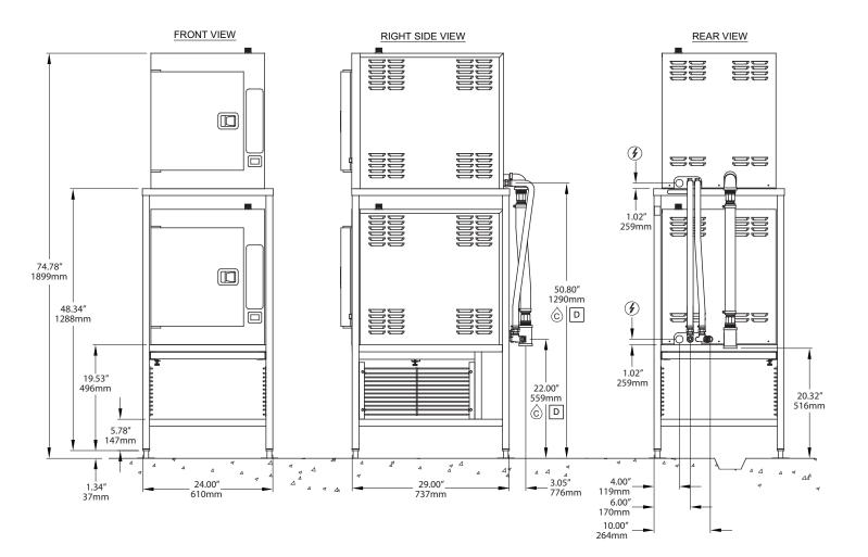
\*NOTES: The diagrams above are shown with the model 21-CET-8 mounted on the ES-2446 Stacking Equipment Stand.
