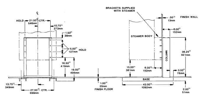
NOTE: Contractor to supply eight, 5%" Studs - Hold Downs for Carrier (as shown on plan view). 16 nuts to be supplied by Contractor for 5%"-11 NC thd. for steamer suspension.
