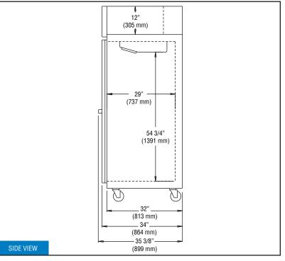
**IMPORTANT NOTE:** If the cabinet is located directly against a wall and/or under a low ceiling, a <u>minimum</u> clearance of 12" is required.
