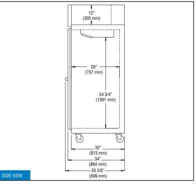
**IMPORTANT NOTE:** If the cabinet is located directly against a wall and/or under a low ceiling, a <u>minimum</u> clearance of 12" is required.
