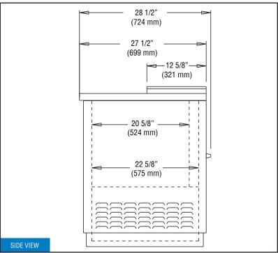
$\underline{\textbf{IMPORTANT NOTE}}\text{: A }\underline{\textbf{minimum clearance of 3" is required}}\text{ on each side, front and rear of cabinet for optimum performance.}$
