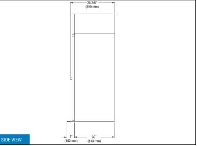
IMPORTANT NOTE: If the cabinet is located directly against a wall and/or under a low ceiling, a minimum clearance of 12" is required.
