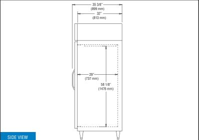
IMPORTANT NOTE: If the cabinet is located directly against a wall and/or under a low ceiling, a minimum clearance of 12" is required.
