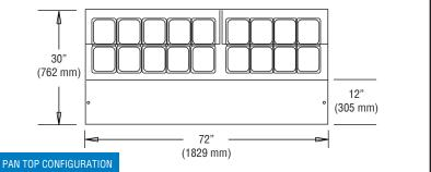
Note: Shown with two tier drawers, see Standard Design Features for drawer pan configurations.
