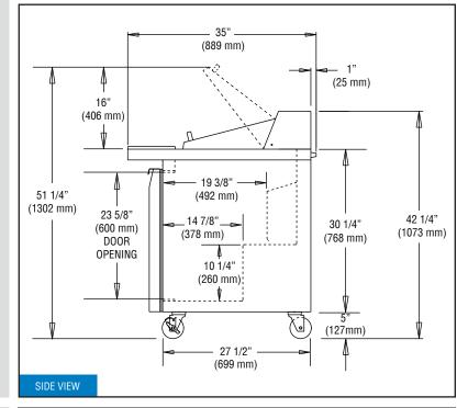
\* Rating @  $+25^\circ$ F evaporator, 90°F ambient Figures in parentheses reflect metric equivalents rounded to the nearest whole unit.
