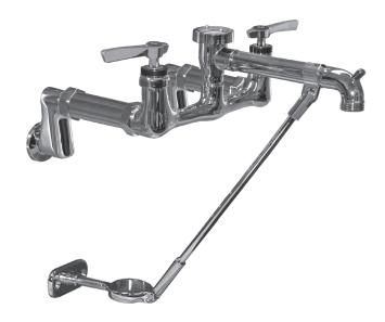
1/2" NPSM Female Inlets Inlets adjustable from 4" (102mm) to 8" (203mm) Operating Temperature: 40 - 180°F (5 - 83°C) Operating Pressure: 15 - 125psi Note: 1-1/8" (29mm) holes for backsplash are recommended to accommodate 1/2" supply nipples.
