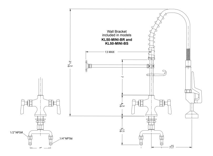
1-1/2" (29mm) hole for deck is recommended to accommodate 1/2" supply nipples.
