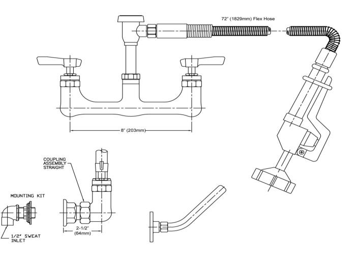
1-1/2" (29mm) holes for backsplash are recommended to accommodate 1/2" supply nipples. 1/2" NPT Male Operating Temperature: 40 - 180°F (5 - 83°C) Operating Pressure: 15 - 125psi
