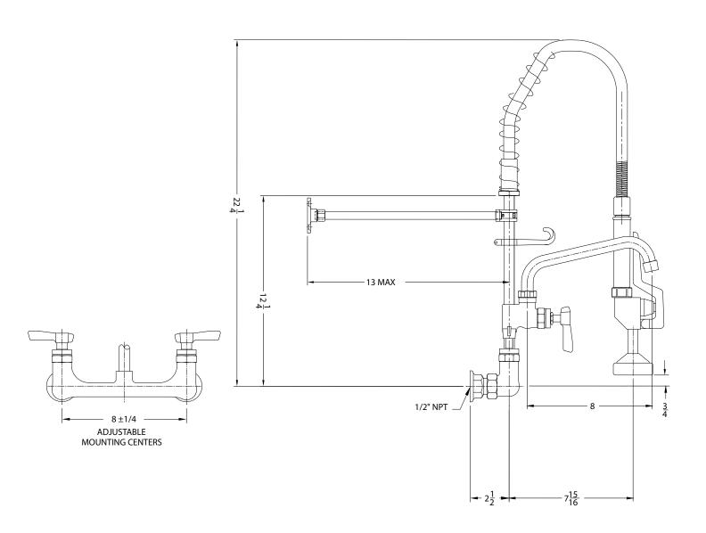
1-1/2" (29mm) holes for backsplash are recommended to accommodate 1/2" supply nipples. 1/2" NPT Female Inlets
