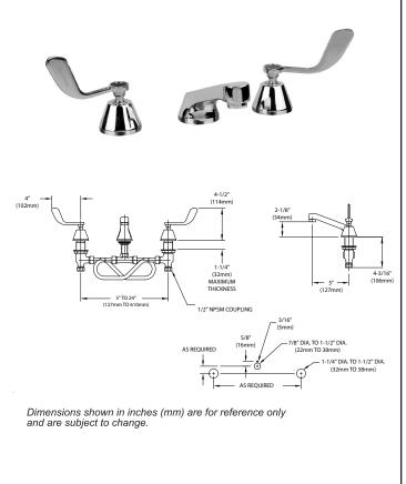
1-1/2" (29mm) holes for deck are recommended to accommodate 1/2" supply nipples.
