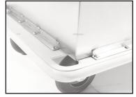
FULL PERIMETER BUMPER... All aluminum with non-marking gray vinyl insert to protect cart and facility walls. Reinforced with angle brackets and bolted on to cabinet. Additional brackets attached to base.
