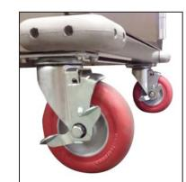
HEAVY-DUTY PERFORMA CASTERS... 5" diameter industrial grade casters with non-marking red rubber cushioned tread. Rust resistant Delrin bearings with all axles and raceways equipped with Zerk grease fittings. Long lasting and easy rolling, yet durable enough to withstand rigorous cart wash programs. Two fixed and two swivel casters with brakes for easy maneuvering.
