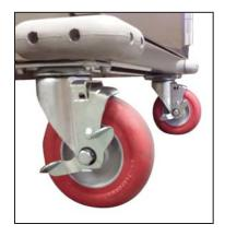
**HEAVY-DUTY PERFORMA CASTERS...** 5" diameter industrial grade casters with non-marking red rubber cushioned tread. Rust resistant Delrin bearings with all axles and raceways equipped with Zerk grease fittings. Long lasting and easy rolling, yet durable enough to withstand rigorous cart wash programs. Two fixed and four swivel casters with brakes for easy maneuvering.
