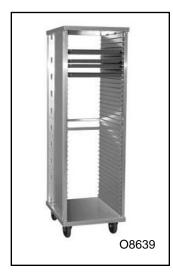
CONSTRUCTION...Heavy-duty, high tensile, all-welded extruded aluminum. Upper frame constructed of vertical uprights 1" x 2.5" x 1/8" thick extruded aluminum channels with top cross and side bracing of 1.25" x 1.25" x .070 wall extruded aluminum tubing, all fully welded together. Solid cap of .063 thick aluminum welded to uprights and cross bracing. Fully reinforced with welded-on horizontal 3/4" x 1" x .070 extruded aluminum stabilizing bars, one at each end.
