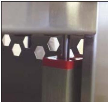
**ULTRA-QUIET RACKS...** with adjustable pin positions to accommodate a variety of tray sizes. Tray spacing fixed on standard 5.75" centers.
