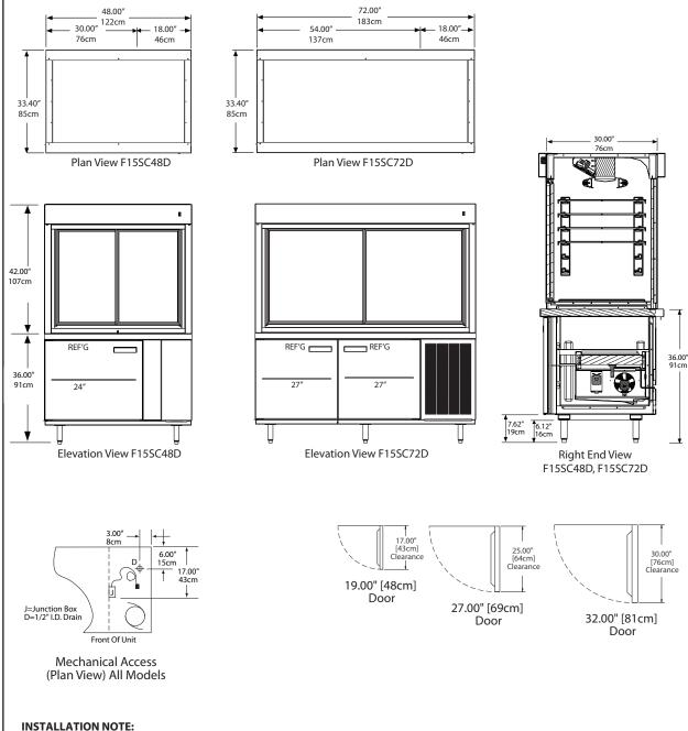
Unobstructed airflow must be maintained to insure unit performance and maintain warranty.
