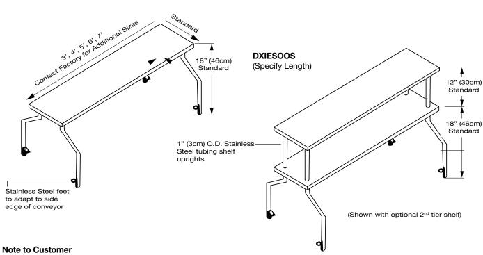
When ordering specify the type of conveyor the shelf is to be used with. If shelf is to be used on an existing conveyor, specify size and type of edge stainless steel feet will be adapting to.
