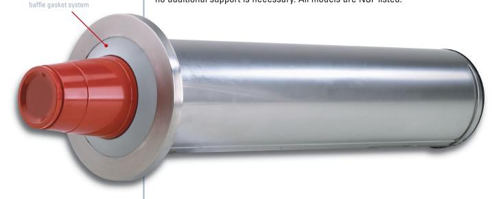
The BFL-2 is a One-Size-Fits-All model that offers maximum dispensing flexibility. This unit is designed to accommodate a variety of 8 oz. to 44 oz. paper, plastic or foam cups with rim diameters ranging in size from 3"–4½". This model comes in two under counter lengths: 22" or 19". The BFL-2 models require a 5½" hole cut-out.
