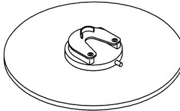
Illustration of underside of a typical mold with horse shoe retainer attached. Retainer fits into index hole on Model No. DP1100M & DP3300M.
