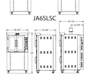
WATER INLET 1/4 NPT ENTRÉE D'EAU 1/4 NPT
