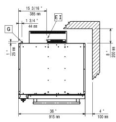
EI=Electrical connectionG=Gas connectionEQ=Equipotential screw
