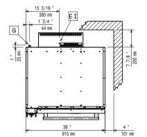
EI = Electrical connection EQ = **Equipotential screw**
