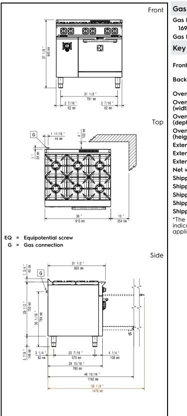
\*The rear and side clearances shown on the diagram indicate the minimum distances reccomeneded from the appliance to combustible surfaces.
