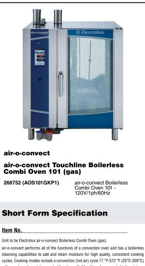
with an automatic moisture control function with 11 settings from zero to high moisture, double step cooking process, automatic pre-heating, a hold function and automatic rapid cooling. All 304 stainless steel construction, seamless hygienic cooking chamber with all rounded corners. Double thermo-glazed door with open frame construction for cool outside door panel. IPX5 (NEMA 4) spray water protection certification.
