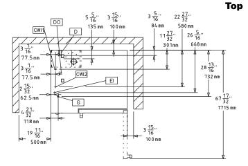
Cold Water inlet CWI = D Drain
