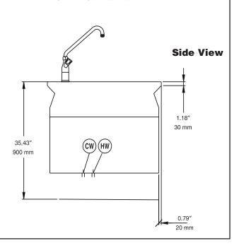
Modular Cooking Range Line S90 Worktop with Water Mixing Unit 4", Island Installation
