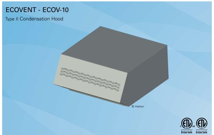
The Halton EcoVent ECOV-10 condensate hood has been designed to fit on Electrolux ovens only (see model chart below) . No direct connection to an outgoing extract system is required, as the steam laden air is filtered by means of baffle filters, mesh moisture eliminators and perforated cassette.
