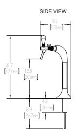
For connection to Elkay **CARBONATION CHILLER** only. Not to be connected directly to main water supply or other chillers Customer to provide mounting hole in countertop. Mounting hole diameter 1-3/8" to 1-1/2". Additional support is recommended for sheet metal or counter tops under 3/4" thick
