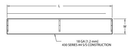
NOTE: BRACKETS SHIP LOOSE SHELF ATTACHES TO BRACKETS WITH SILICONE OR CONSTRUCTION ADHESIVE
