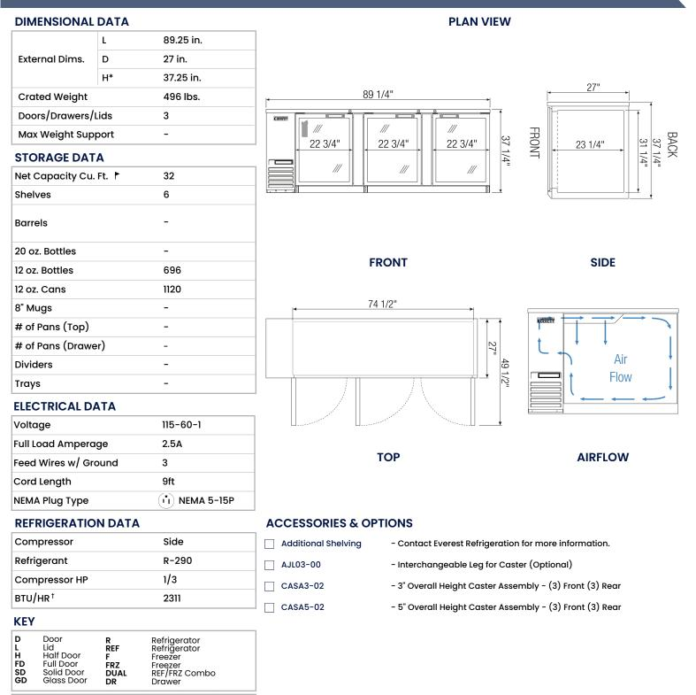
(†) Based on evaporating temperature of 23°F (-5°C) & condensing temperature of 131°F (55°C). () Product capacity is calculated based on standard industry figures. (\*) Reference plan view for clarification on caster/unit height. If dimensions and capacity are critical, please contact Everest Refrigeration. Blizzard R290 replacement is at the sole discretion of Everest Refrigeration. Specifications subject to change without notice.
